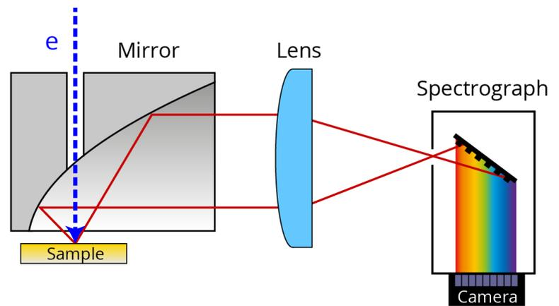
Figure 1 Schematic representation of the hyperspectral imaging mode.
