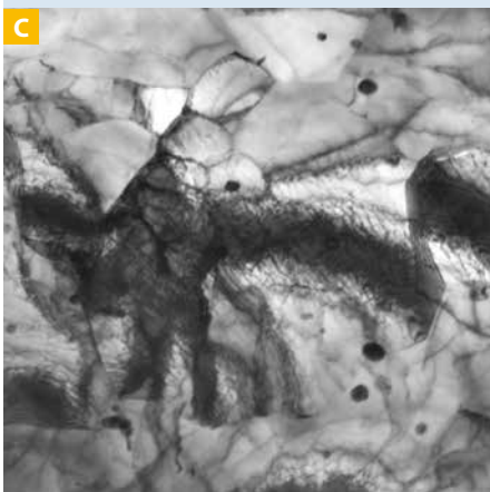
C Dislocations in a low-angle grain-boundary (aluminium)
